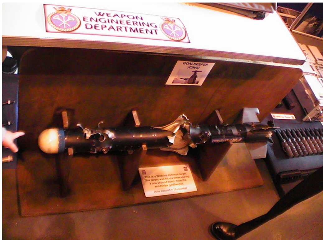
A target hit by Goalkeeper; this target was hit six times during a one-second burst of 70 rounds.
