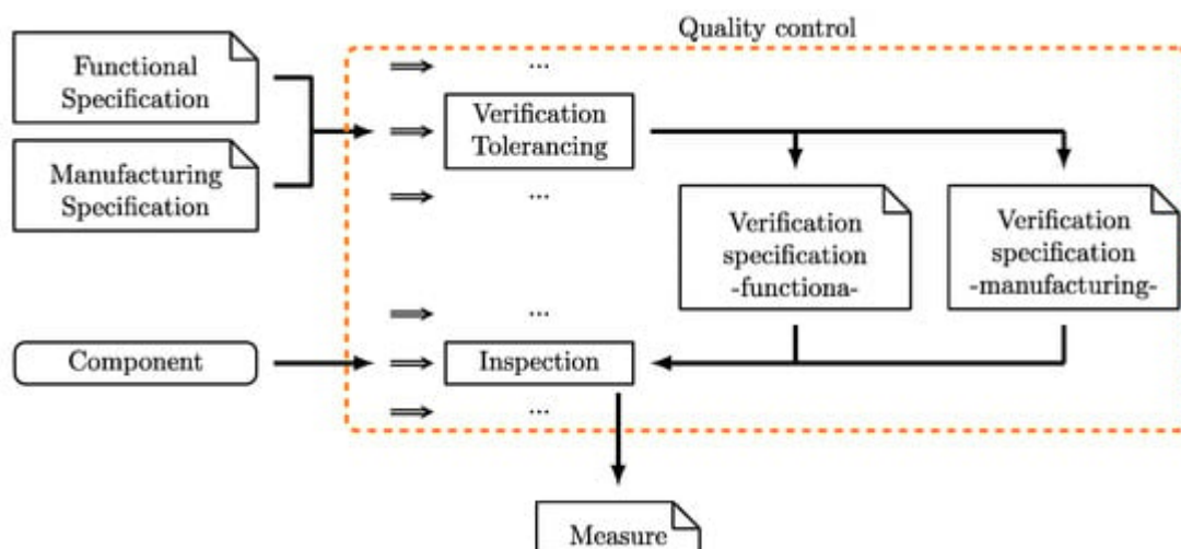
Figure 3. Input/output diagram that describes the verification tolerancing activity taking place inside the quality control department. Other tasks performed by the quality control department are omitted.
