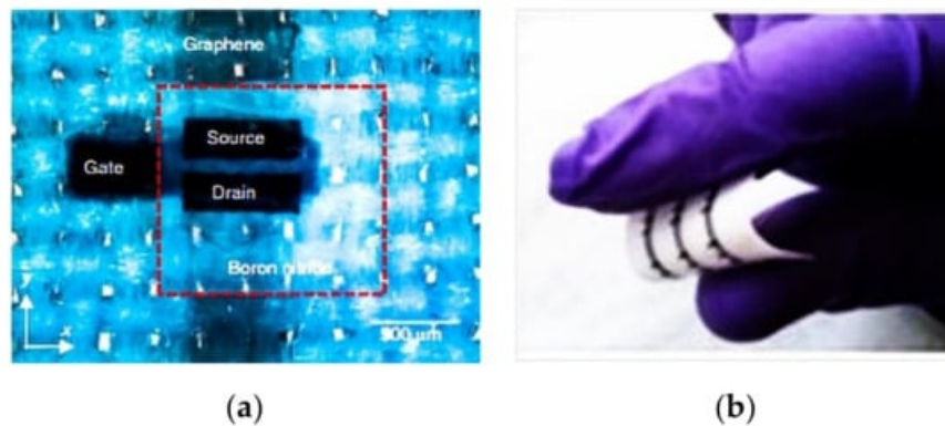
Figure 10. Graphene based biocompatible electronics. Optical microscopy image of the inverted FET on polyester (a) . Image of an array of FETs on textile (b) , reprinted with permission from ref. [133]. Springer Nature http://creativecommons.org/licenses/by/4.0/ accessed on 13 July 2021.
