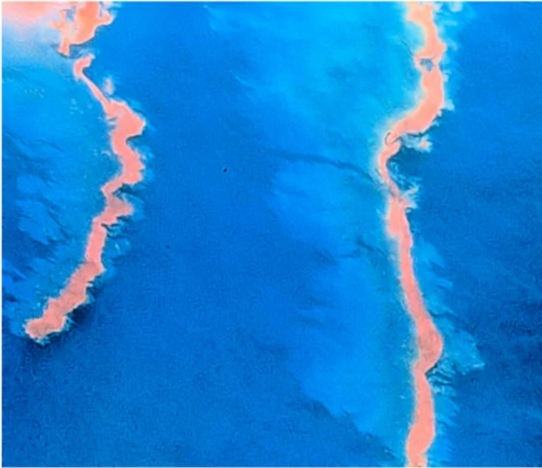
Figure 3. Photograph showing emulsion streaks surround by sheen (thin oil). This photograph was taken from an aircraft flying at about 1000 m.
