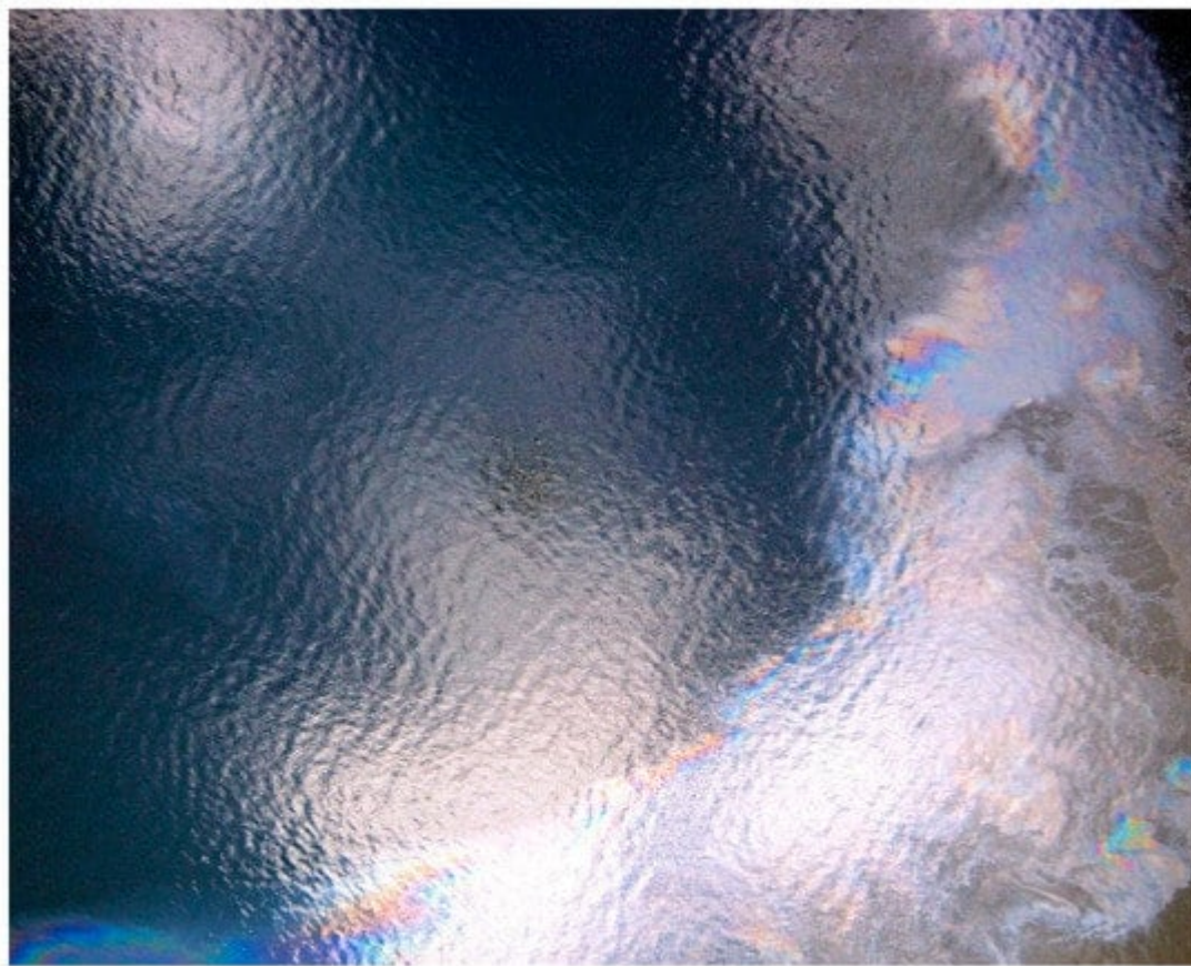
Figure 1. A photograph of a rainbow sheen taken from an aircraft at an altitude of about 300 m. This color of sheen has a strong physical relation to 1 to 1.5 \mu\text{m} .
