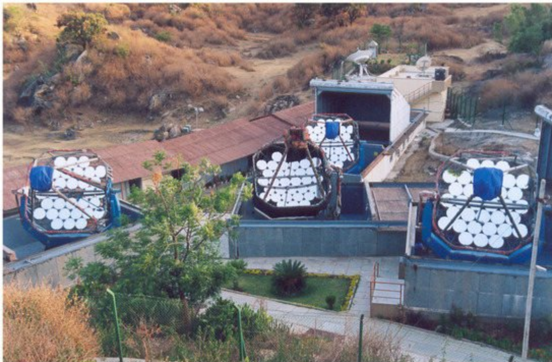
Figure 1. The TeV Atmospheric Cherenkov Telescope with Imaging Camera (TACTIC) telescope array operational since 2001 at Mount Abu, India. Single telescope at the center is being used as an imaging unit for TeV \gamma -ray observations.
