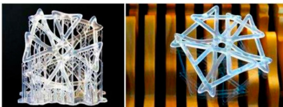
Figure 7. The use of 3D printing enables the production of parts that cannot be made in any other fashion, 10 cm by 10 cm test prints [37].
