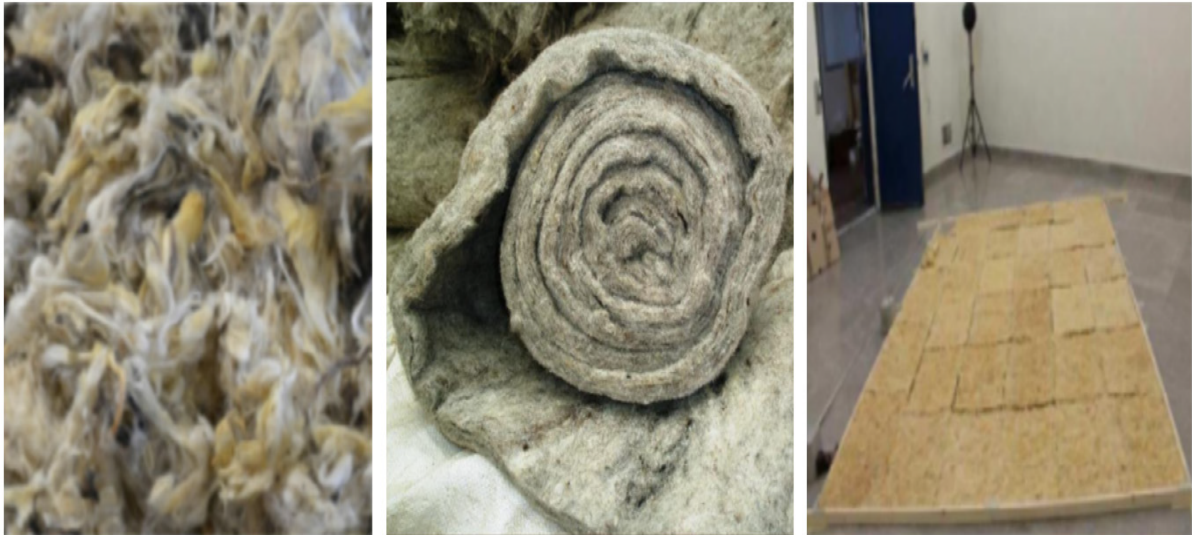
Figure 4. Applications of sheep wool insulation in building constructions [7][9].
