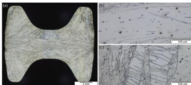
**Figure 4.** Microstructure of an AZ31 variation (AZ31 containing 0.3Ca and 0.2Y) in as-forged condition, formed at 425 °C stock temperature and 280 °C die temperature at a ram speed of 10 ms<sup>-1</sup>, showing (a) cross-section of forged part, (b) sample center, (c) sample rim.
