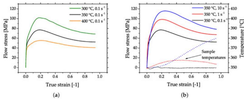
**Figure 3.** Flow curves of cast and homogenized AZ31, obtained by cylinder compression testing. The plots show the flow stress (full lines) of samples tested with (a) varying temperatures and (b) varying strain rates. The dotted lines in (b) show the increasing sample temperatures with increasing strain rate. No temperature compensation was done for the shown flow stress values.
