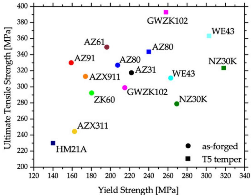
**Figure 5.** Tensile properties of various Mg alloys, showing as-forged and artificially aged (T5) values at room temperature (RT). The graphic shows mean values calculated from various scientific sources.
