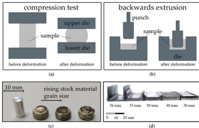
**Figure 2.** Schemes of simplified testing set-ups for (a) compression testing and (b) backwards extrusion; (c) AXM lean alloy compression samples with varying stock material grain sizes tested at 400 °C. Picture (d) shows parts manufactured from AZ31 by backwards extrusion at 250 °C with varying forming load<sup>[3]</sup>, reproduced with permission from Elsevier.
