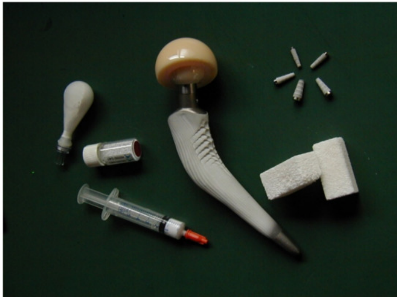
Figure 1. Several examples of the commercial \text{CaPO}_4 -based bioceramics.
