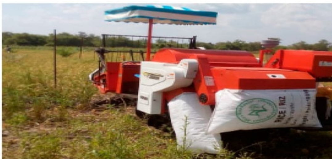
Figure 11. Collection of grain losses in a woven sack at the rear and concave of the machine [41].
