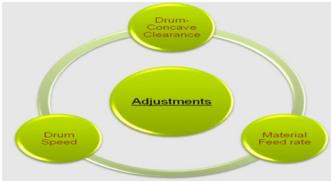
Figure 3. Machine parameters that affect threshing and separation losses.
