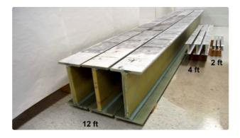
Scaled composite laminated I-beams with different scales and lamination schemes designed based on structural similitude analysis. https://handwiki.org/wiki/index.php?curid=1493497
