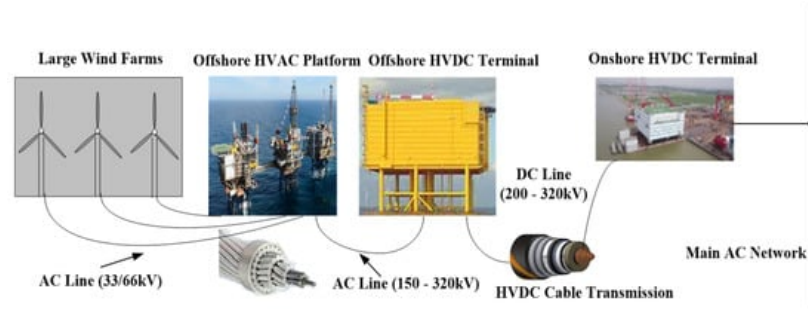
Figure 1. Typical scenario for using HVDC technology to connect offshore wind power to the main AC network.
