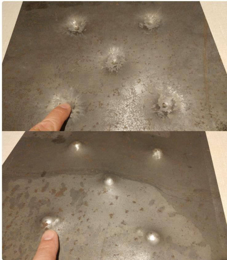
Swebor-brand high-strength low alloy steel plate, showing both sides, after plastic deformation from defeating projectiles in ballistics testing. Note: When exposed to fire, steel first expands and then loses its strength, exceeding critical temperature at 538°C or 1000°F per ASTM E119 unless treated with fireproofing. <https://handwiki.org/wiki/index.php?curid=1403964>
