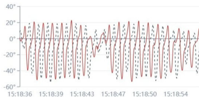
Figure 1. The angle curve of leg flexion and extension in the vertical direction during walking. The red line represents the left leg, and the black dotted line represents the right leg.
