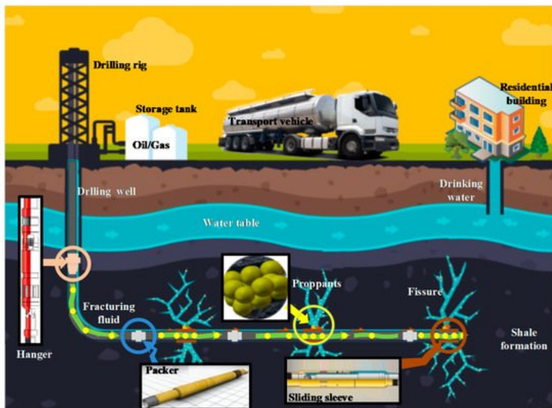
Figure 1. Schematic of the hydraulic fracturing process.
