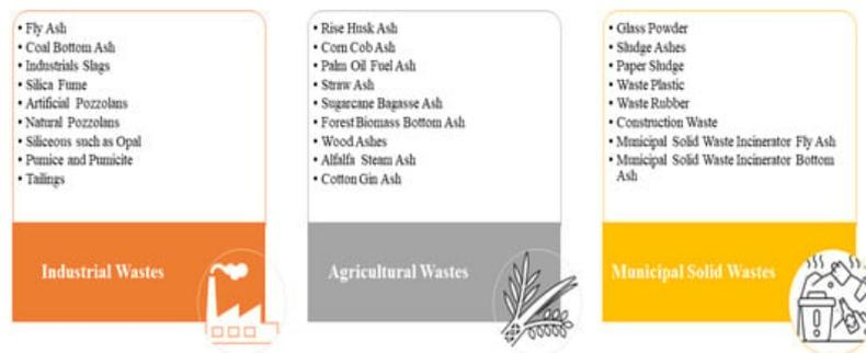
**Figure 1.** Solid wastes incorporated into geopolymers as potential aluminosilicate precursors.
