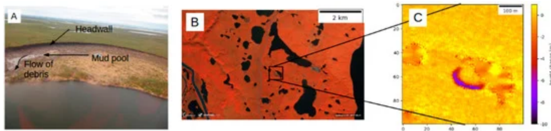
Figure 11. Mackenzie River Delta, Canada: (A) Aerial snapshot of a thaw slump. (B) Sentinel-2 L1C. Image containing the slump in August 2017. (C) Digital elevation model (DEM) processing results after single-pass TanDEM-X observation in June 2015. Source: ETH Zurich.
