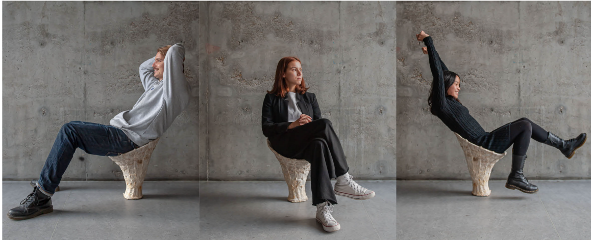
Figure 5. Seating tests up to 90 kilos.
