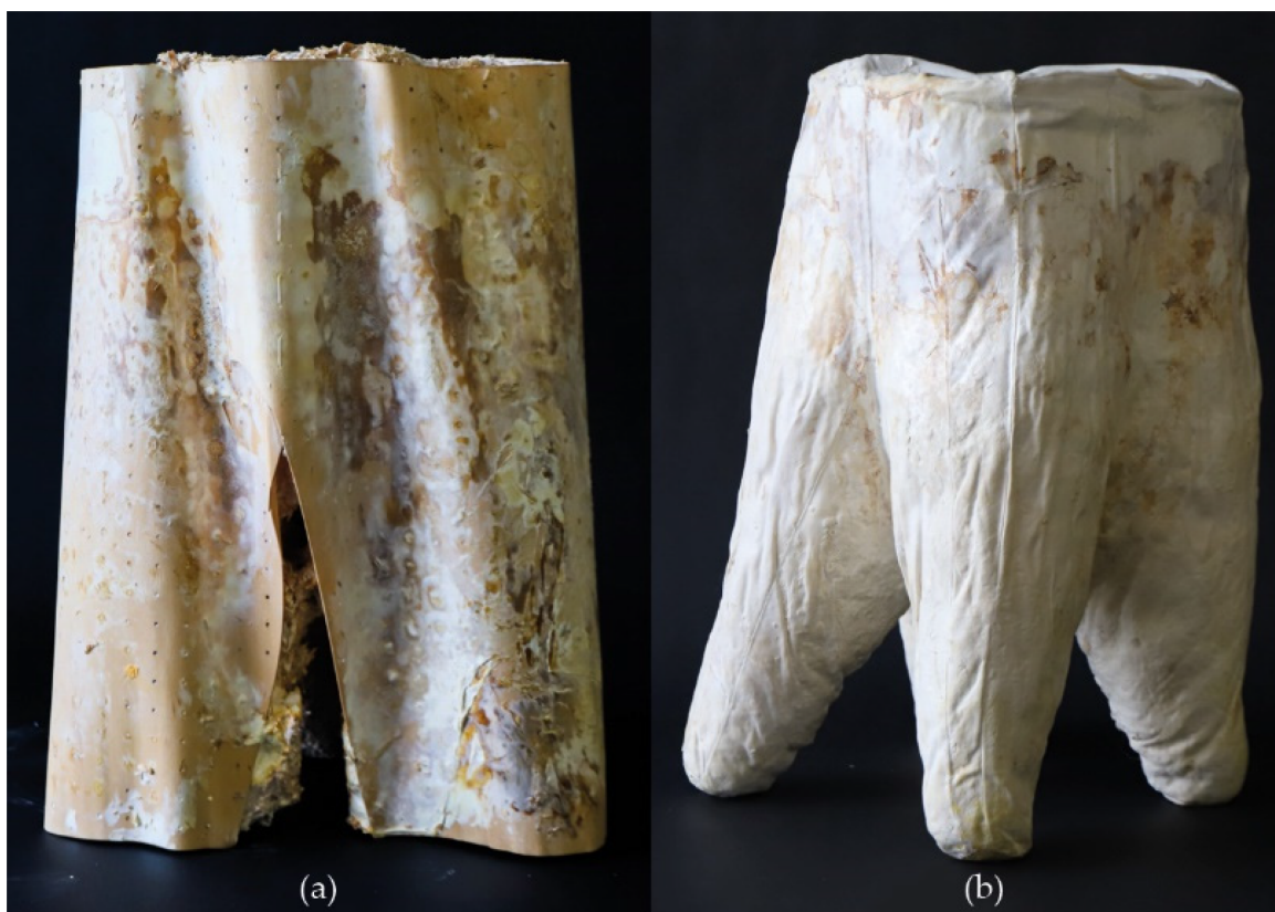
Figure 1. Results of grown on different skin materials: (a) hemp sheets, (b) jute sheets, (c) knitted hemp rope.
