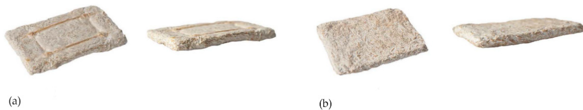
Figure 2. (a) Results of multilayer composite, (b) hemp mat sandwich.
