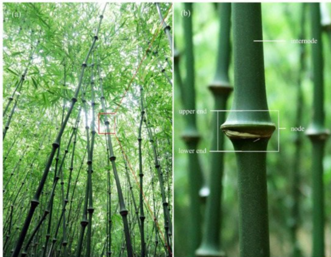
Figure 1. Preparation of \mu CT sample. (a) Bamboo. (b) Sampling location (white wireframe area).
