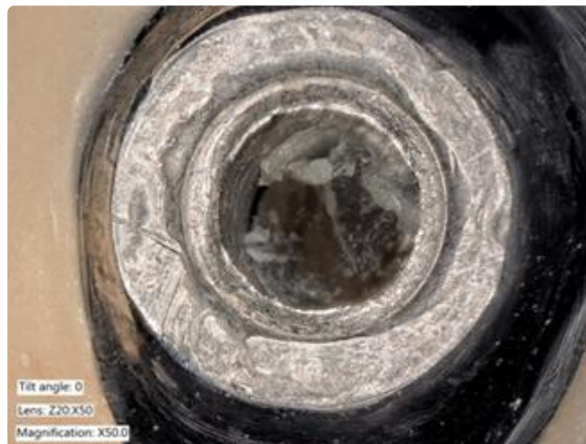
Figure 13. Evaluation of the basal aspect of the implant crown, showing deformation of the hexagon, and particle delamination.
