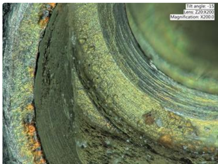
Figure 9. Closer view of an explanted implant with a hexagonal connection. Corrosion, delamination, and abrasions of the connection surface can be appreciated.
