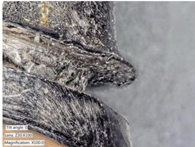
Figure 12. Corrosion of the abutment can occur and appears as pits, or color changes (dark, brown or yellow) distinguishable from the natural gray color of the implant.
