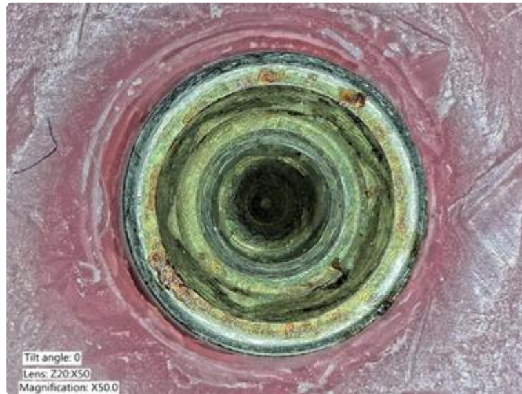
Figure 8. Explanted implant with a hexagonal connection. The implant crown was removed. The implant connection at microscope evaluation showed wear, signs of corrosion, and titanium particles.
