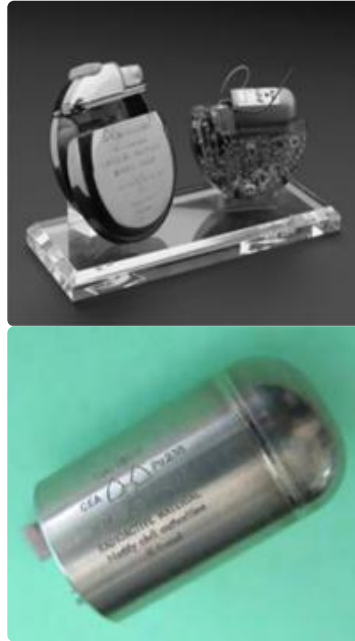
Figure 4. Left pacemaker and right RTG battery [21].
