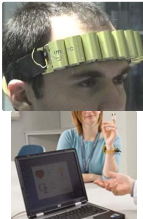
Figure 8. (a) TEG supplies power to an EEG system mounted on an expandable headband [46] ; (b) Wireless pulse oximeter [47]
