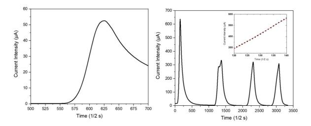
Figure 2. Temporal evolution of effective current intensity in the clinoptilolite sample with the turning on/off of the heat source (a) and NTC material behavior under repeated thermal pulses (b). Linearity of the temporal current intensity behavior is shown in the inset.
