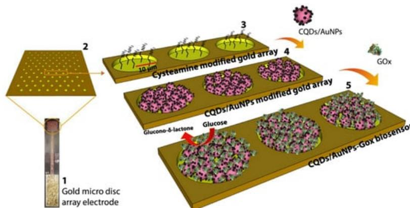
**Figure 3.** Preparation steps of a glucose biosensor using a micro disk array electrode. (1) single disk array electrode, (2) surface magnification, (3) cysteamine modification of the Au surface, (4) CQDs/AuNPs adhered surface, (5) GOx immobilisation to the surface [113].
