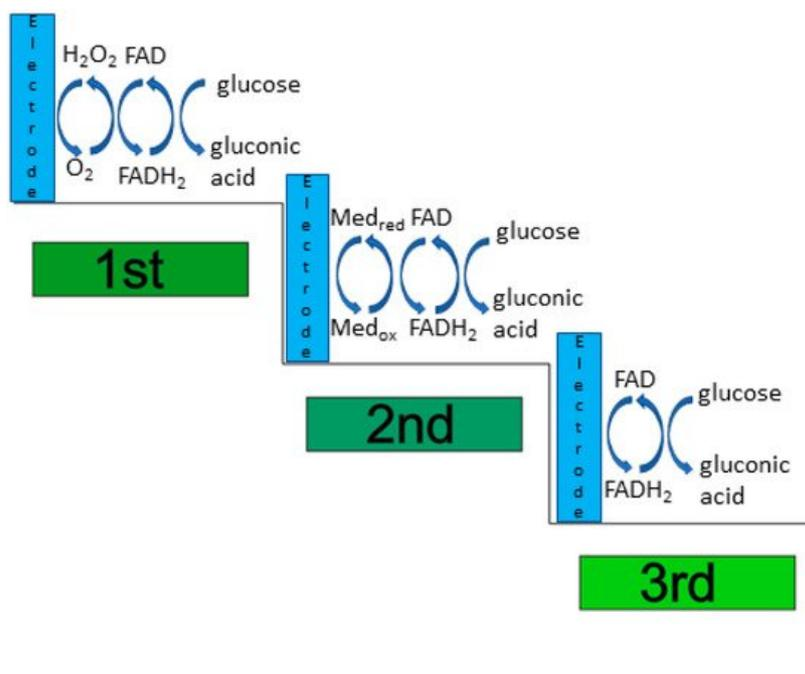
**Figure 2.** Schematic representation of enzymatic glucose oxidation mechanisms for the three different generations of biosensors.
