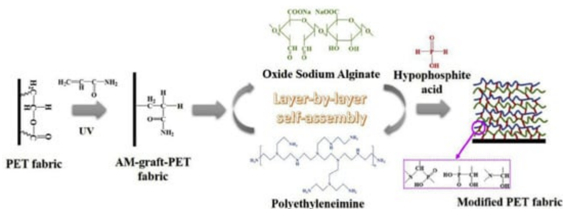
Figure 5. Schematic of LbL deposition of pre-treated MA-graft-polyester (PET) fabric coated with 15 BLs of OSA/PEI and post-treated with HA cross-linking [62] Reproduced with permission from Pan, Y.; Liu, L.; Song, L.; Hu, Y.; Wang, W.; Zhao, H., Polym. Degrad. Stab. ; published by Elsevier Ltd., 2019.
