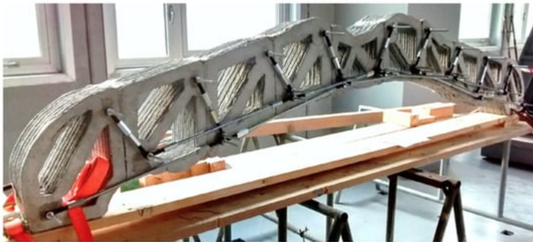
Figure 5. Printed hollow concrete units assembled and reinforced by external steel rebars [52].
