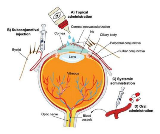
**Figure 1.** Schematic representation of the human eye and routes of administration for preclinical corneal drug delivery. (**A**) Noninvasive topical administration (eye drops), (**B**) subconjunctival injection given underneath the conjunctiva lining the eyelid, (**C**) systemic administration as intravenous injection, intraperitoneal injection or implanted osmotic pump, and (**D**) oral administration (gavage).
