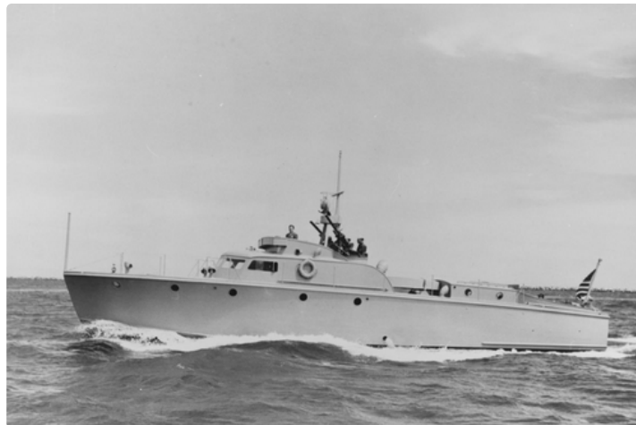
US Navy NH 96504 a 63 ft (19 m) air-sea rescue boat built by Fellows & Stewart. https://handwiki.org/wiki/index.php?curid=1100329
