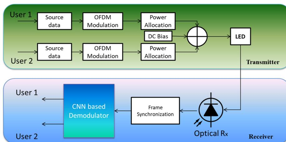
**Figure 6.** An overview of NOMA-VLC system using a CNN-based demodulator.
