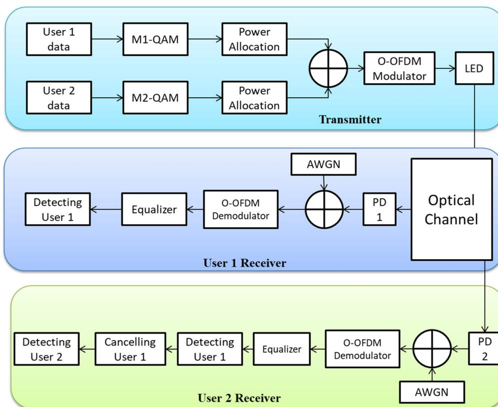
Figure 5. Block diagram of two-user NOMA-based VLC system with QAM and O-OFDM.
