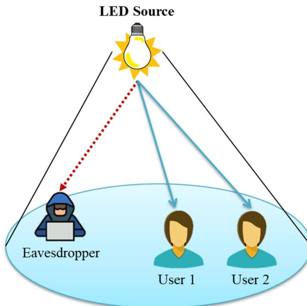
**Figure 7.** NOMA-VLC system with two users and an eavesdropper.
