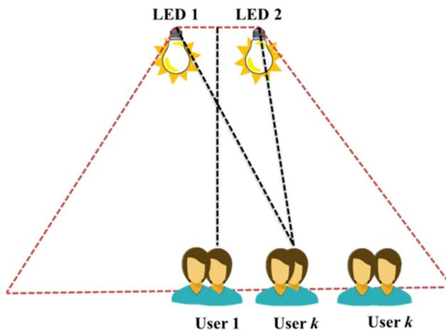
**Figure 1.** An overview of  $2 \times 2$  MIMO-NOMA-based VLC system with  $k$ -users.
