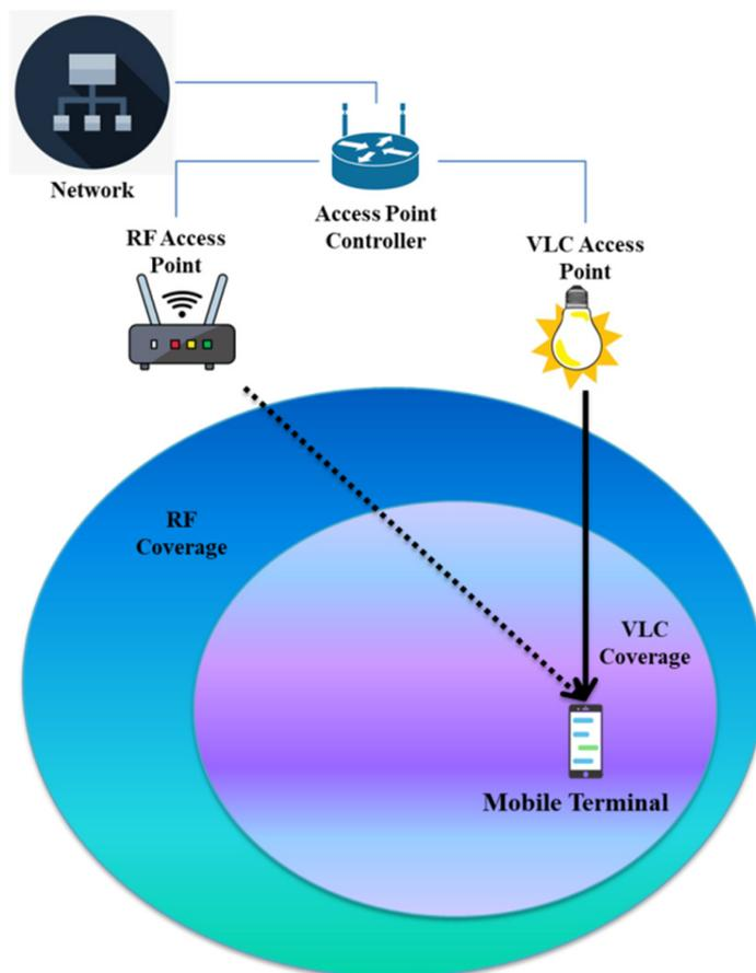
**Figure 3.** An overview of Hybrid RF/VLC wireless network.
