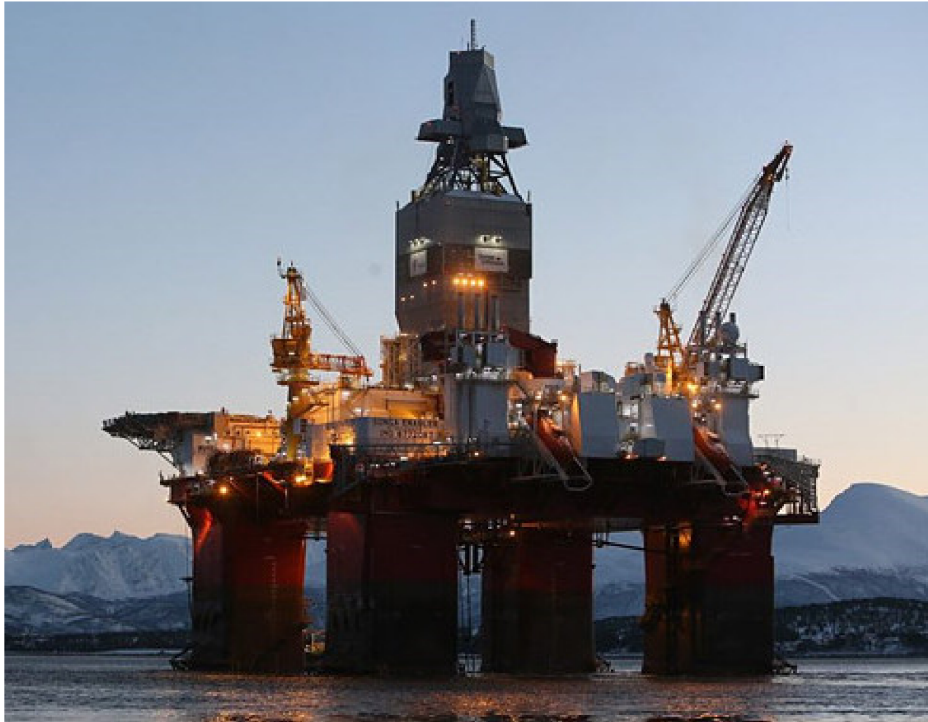
Figure 4. Transocean Enabler semi-submersible drilling rig built in 2016 and designed to operate in harsh environments (Courtesy: Transocean).
