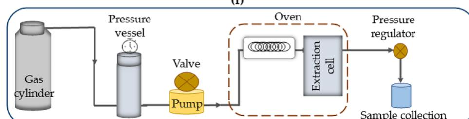
**Figure 2.** Simplified representation of the most used green extraction procedures, (a) supercritical fluid extraction, (b) subcritical water extraction, (c) pulsed electric fields, (d) ultrasound-assisted extraction, (e) microwave-assisted extraction, (f) enzyme-assisted extraction, and (g) pressurized liquid extraction.
