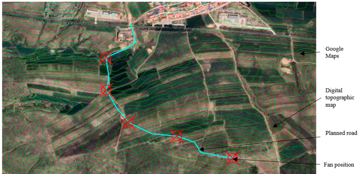
Figure 3. Path design on a digital topographic map.
