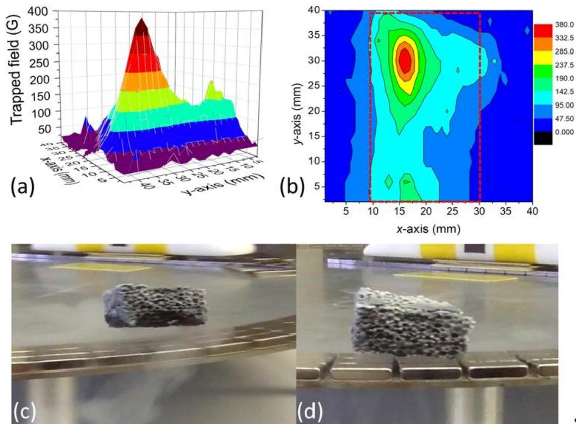
**Figure 3.** Trapped field measurements on a foam sample. Distribution of  $B_z$  measured by scanning Hall probe on different sample sides of the foam as surface plots (a,c) and contour plots (b,d). The sample position is marked in the contour plots by a dotted red line. Superconducting foam levitating above a magnetic rail. (a) shows the foam sample at full speed running on the rail, and (b) gives the foam sample when being close to warm up.
