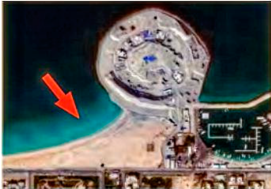
Figure 1. Interruption in natural sediment drift: the red arrow on the left indicates the increased sedimentation that might modify the natural shape of the shoreline (Source: Umm Suqeim 2 Harbor 25°09'08.01" N and 55°11'50.46" E) [32].
