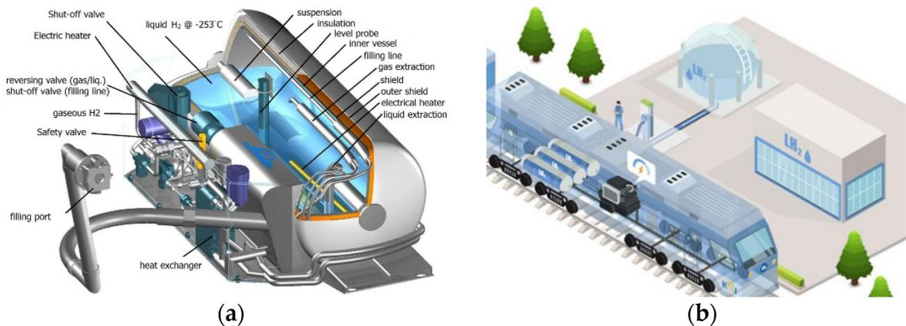
**Figure 4.** (a) Liquid hydrogen storage system from Linde [23]; (b) Schematic of the LH<sub>2</sub>-hybrid train and the charging infrastructure presented by KRRRI.
