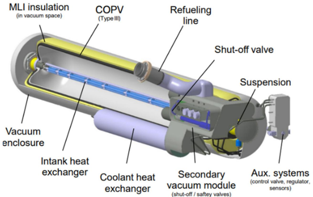
**Figure 5.** Schematic of CcH<sub>2</sub> storage vessel from BMW.
