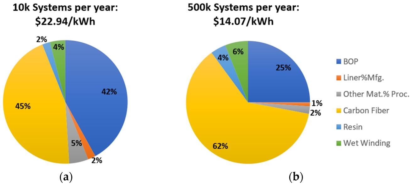
**Figure 1.** Cost breakdown for type IV 700 bar H<sub>2</sub> single tank storage systems with 5.6 kg usable (from DOE): (a) 10 k systems per year; (b) 500 k systems per year [5].
