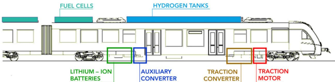
**Figure 2.** Diagram of Coradia iLint train, Alstom, propulsion system [\[12\]](#).
