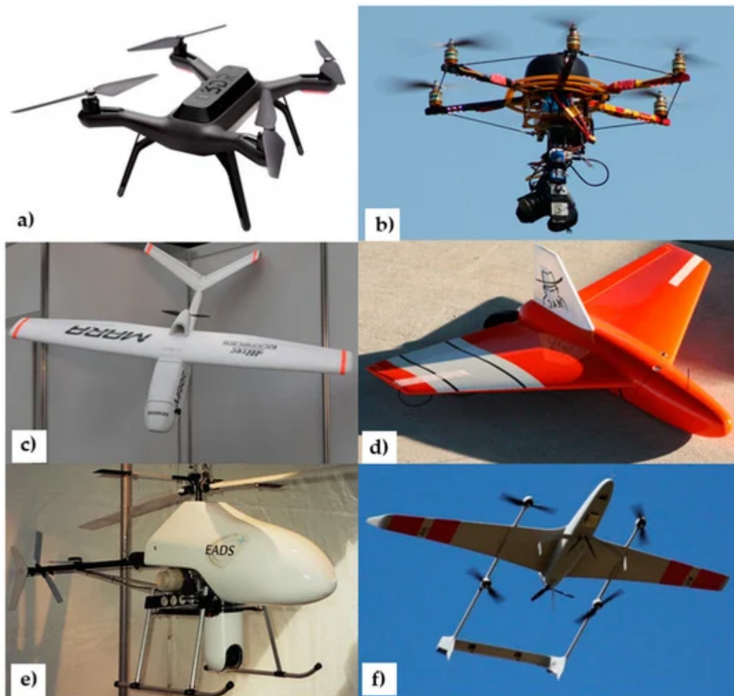
Figure 1. Unmanned aerial vehicle (UAV) types for remote sensing civilian usage: rotary-wing (a,b), fixed-wing (c,d), unmanned helicopter (e), and hybrid solution (f).
