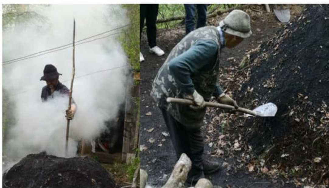
Figure 3. Carbonization process monitoring by the operators: on the left, the operator controls the ignition of the charcoal pile; on the right, the operator covers the base of the charcoal pile with earth to prevent air entrance.
