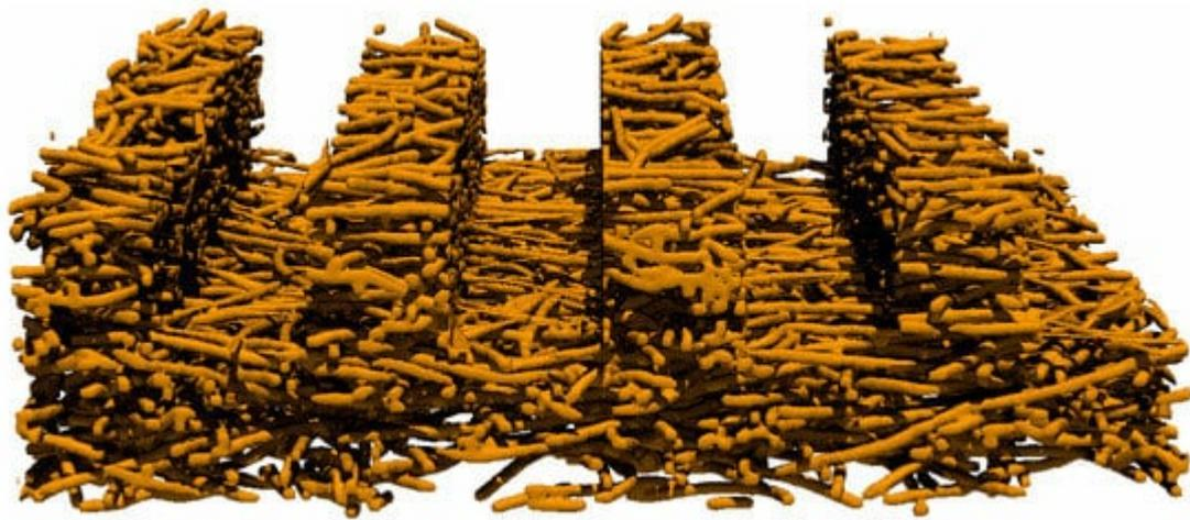
**Figure 1.** Illustration of a combination of straight line microchannels above the fibrous porous structure.
