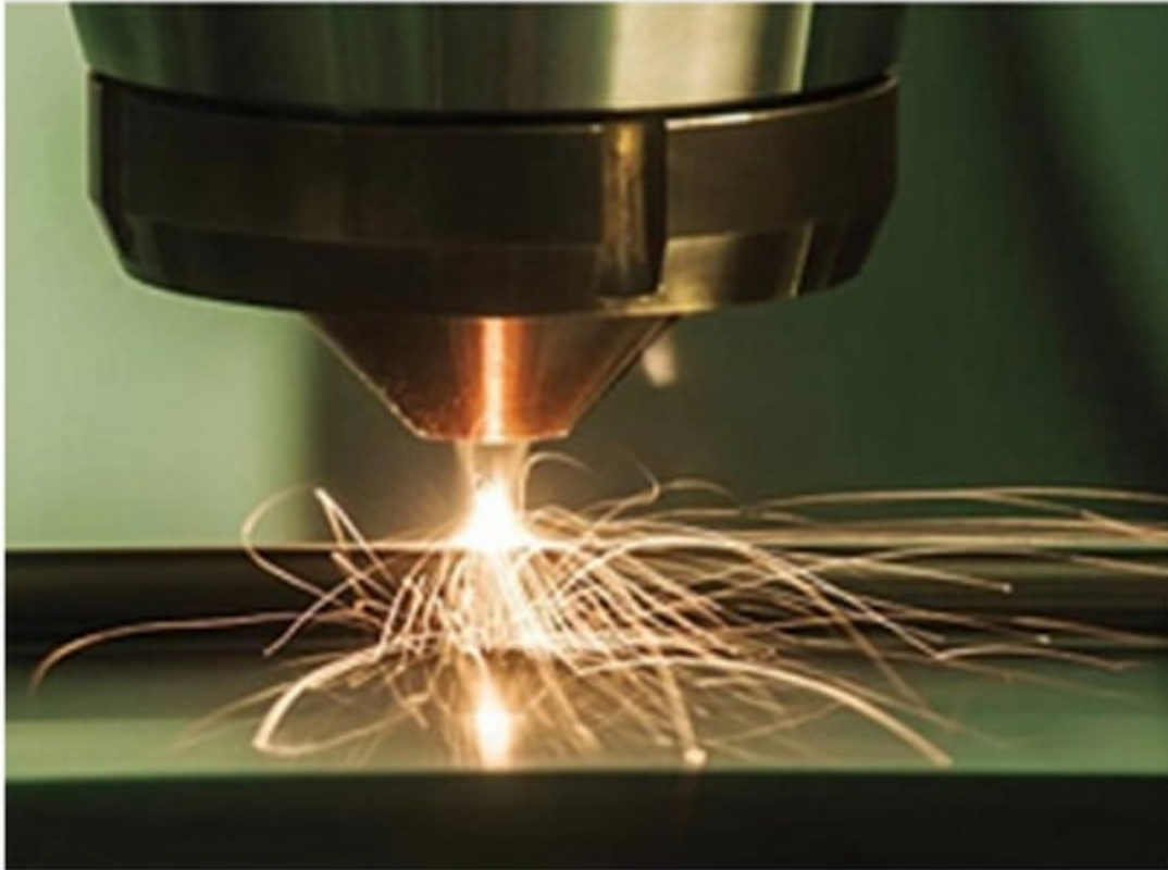
Figure 7. Illustration of a laser-powered DED process [46] .
