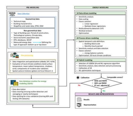
Figure 1. Methodology of USBEM using a place-based approach.
