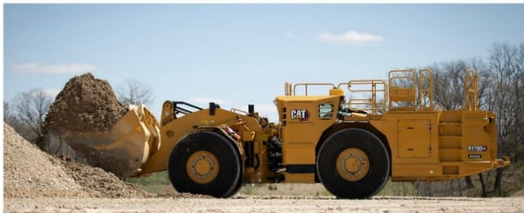
Figure 3. Caterpillar R1700 XE LHD which uses battery-powered electric motors for propulsion [27] .
