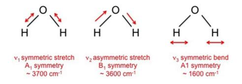
Figure 4 – Fundamental modes of vibration of a free water molecule.
