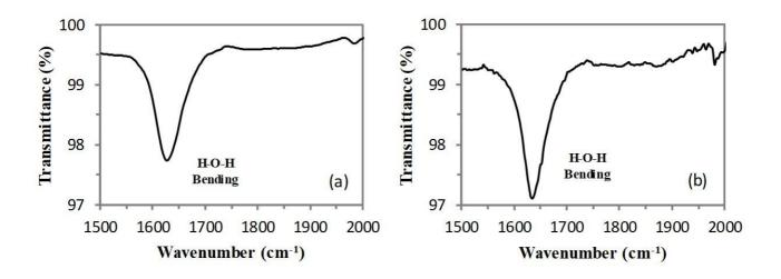
**Figure 5** – FT-IR of clinoptilolite in the 1000-2000cm<sup>-1</sup> spectral range before (a) and after (b) the thermal treatment.
