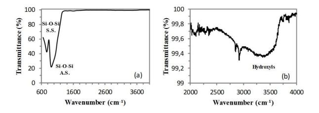
Figure 1 – FT-IR spectrum (in ATR mode) of an optical microscope slide.
