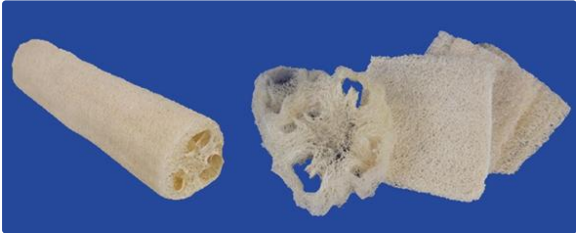
Figure 2. Luffa and its internal structure.
