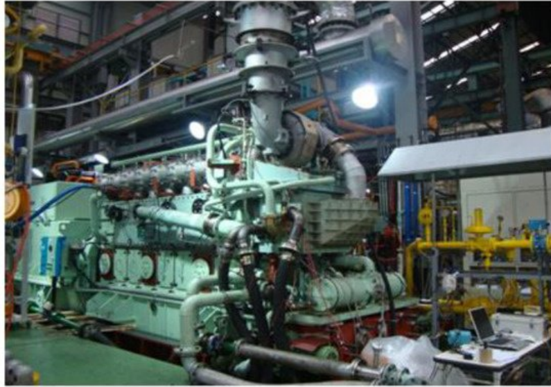
Figure 3. Photograph of the gas engine developed in this study.
