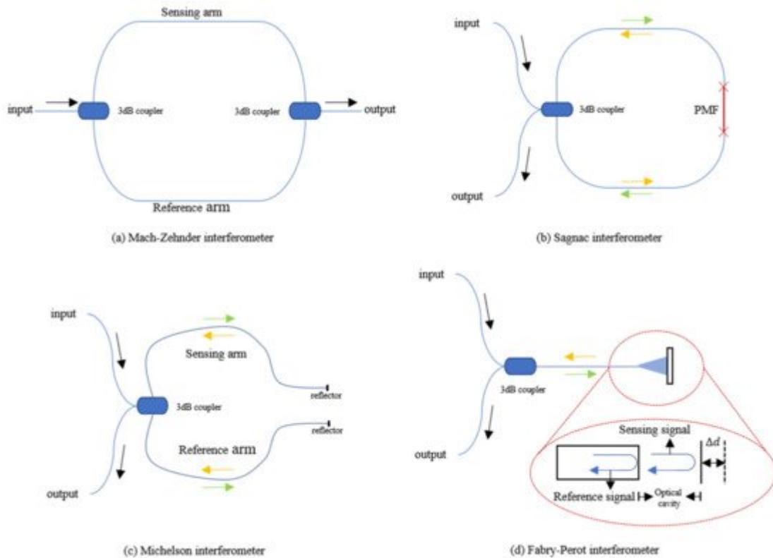
**Figure 1.** (a) Structure of optical fiber Mach–Zehnder interferometer; (b) Structure of optical fiber SI based on PMF; (c) Structure of optical fiber Michelson interferometer; (d) Structure of optical fiber Fabry–Perot interferometer.
