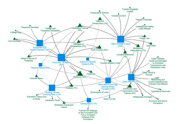
Figure 1. Graphical relationship of EPG faults and causes.
