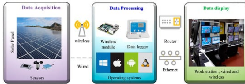
Figure 3. The basic architecture of a solar PV monitoring system.
