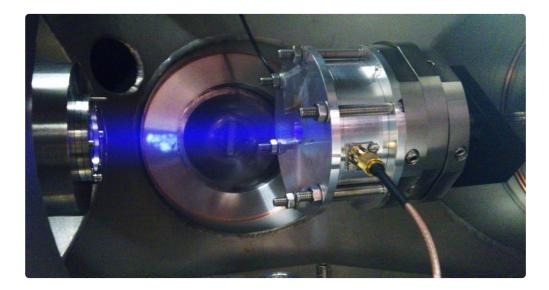
**Figure 1.** Visible light emitted by an EUV-induced plasma. At the right, a resonant cavity is used to measure plasma properties with a technique called Microwave Cavity Resonance Spectroscopy (MCRS).
