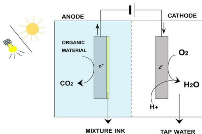
**Figure 1.** Schematic overview of photoelectrochemical cell.
