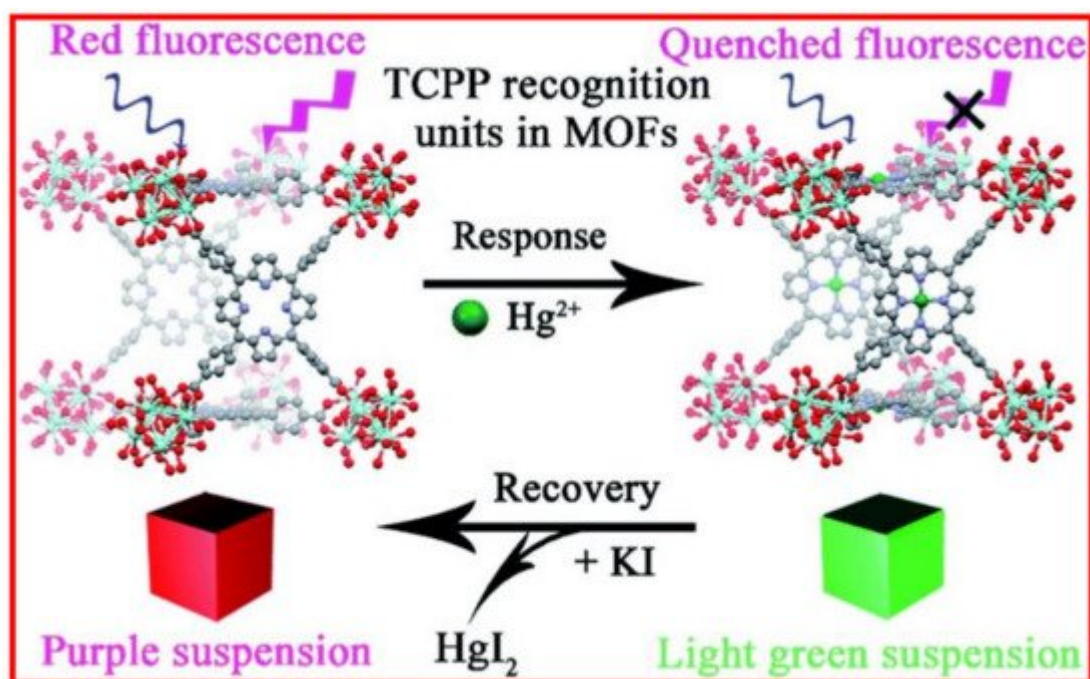
Figure 2. Illustration of the sensor construction protocol. The inherent TCPP linker was designed as the recognition site as well as the signal reporter for \text{Hg}^{2+} sensing at the same time. Upon the addition of solution into the PCN-
