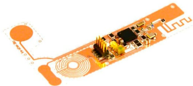
Figure 2. Bluetooth sensor circuit mounted on a flexible substrate. Source: https://www.edn.com/product-how-to-build-your-own-designs-on-flexible-circuit-boards (accessed on 20 March 2021).
